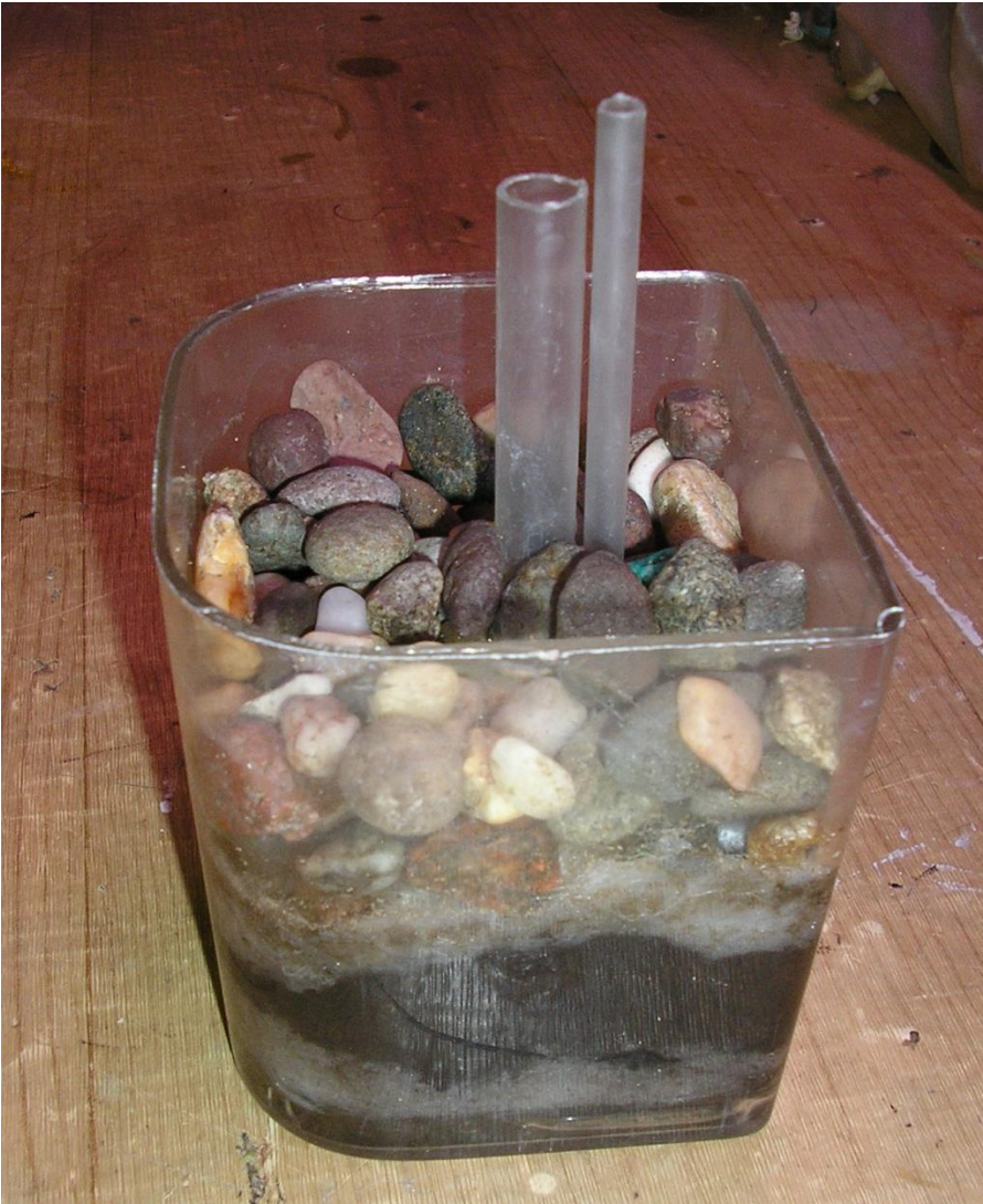
Box filter with peat moss to soften water
